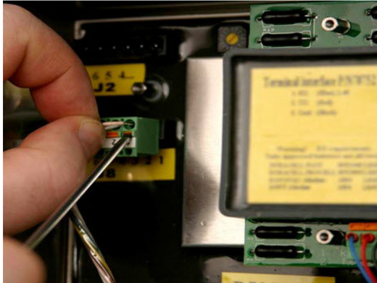
Figure 4-2: Cable termination inside the logger
